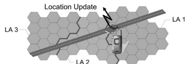
**Fig. 7** Example of location updating on entering a new LA
