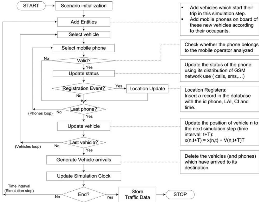
Fig. 6 Basic flow chart of the simulation process
