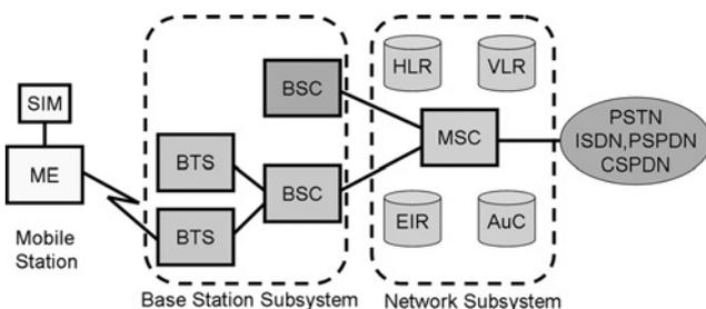
**Fig. 3** Schematic view of the GSM system
