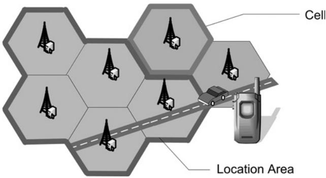
**Fig. 2** Schematic view of several LAs sub-divided into cells
